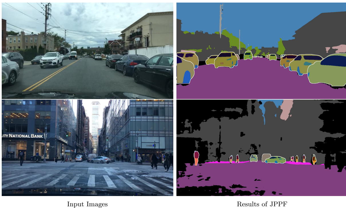
Fig. A4: Visual results of our JPPF on the BDD100K dataset [60] without fine-tuning. The second example shows a failure case, in which our model is not able to properly generalize to the unseen data
